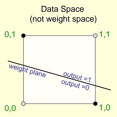
The positive and negative cases cannot be separated by a plane
